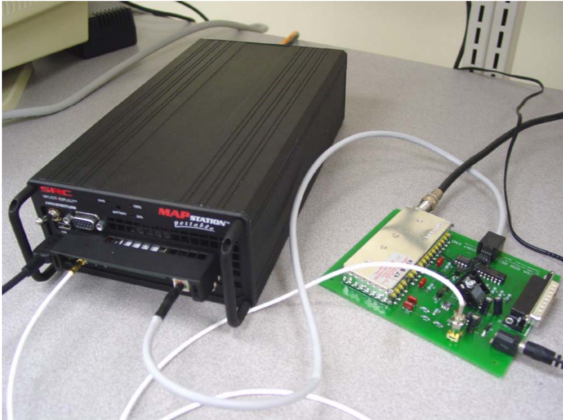
Figure 5. SRC Portable MAP with wide-band RF front-end board.
