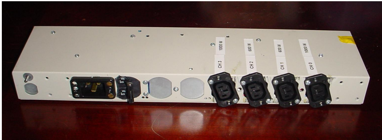
Figure 1. Custom-made power monitoring system.
