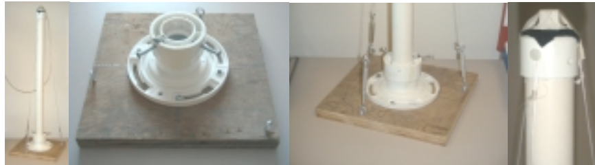
Fig. 2. Assembled sensor holder, wooden platform, and sensor attachment.
